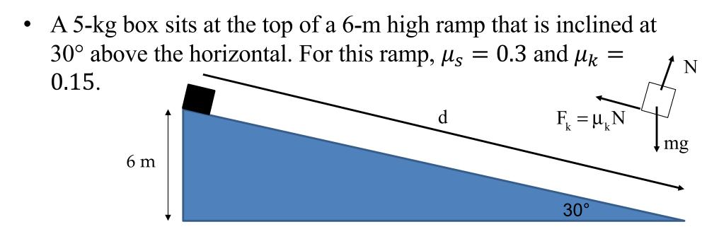
How fast is the block traveling when it gets to the bottom of the incline?
