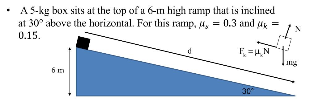
Assuming it slides, how much work is done by each force acting on the box by the time it reaches the bottom of the ramp? Also, what is the net work done during the motion?
